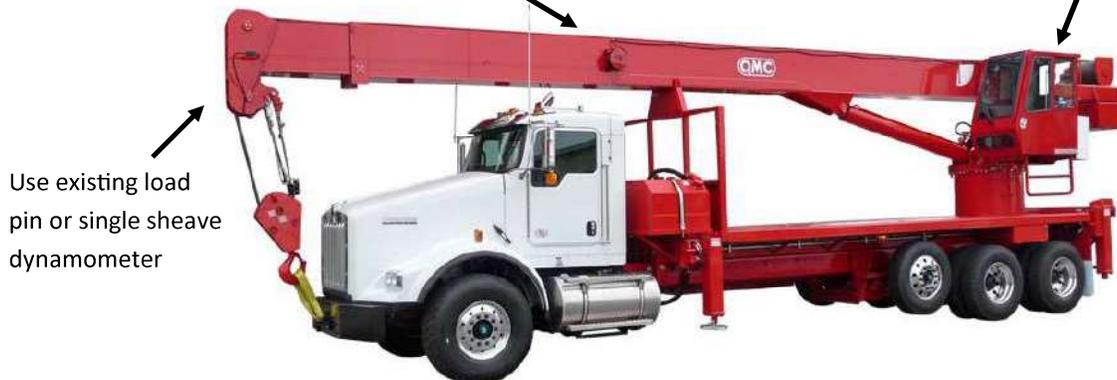
Use existing load pin or single sheave dynamometer
