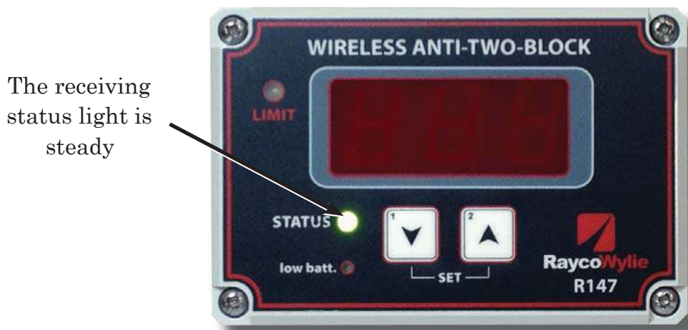
Fig. 4: R147 Normal Mode of operation (no two-block)
