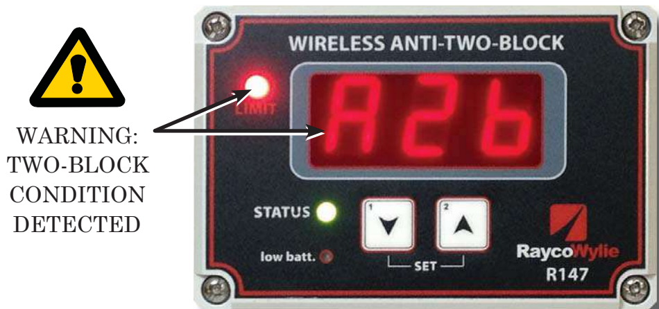
Fig. 5: R147 in a Two-Block condition
