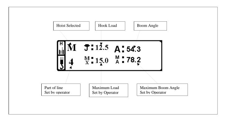
The top row of the display window shows Selected Hoist, Hook Load and Boom Angle. The bottom row shows the Parts of line selected, the maximum Load and the maximum Boom Angle set by the operator.
