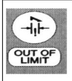
This light will illuminate when a preset limit has been reached. These can include high/low angle, maximum / minimum length, maximum radius, maximum height. A warning message will alternate with the normal screen.
