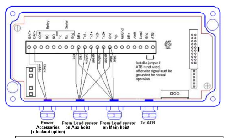
The lockout connection is according to your lockout configuration. Normal operation without ATB alarm gives a relay status of COM-NO. When an ATB condition is detected, the relay status will change for COM-NC.
