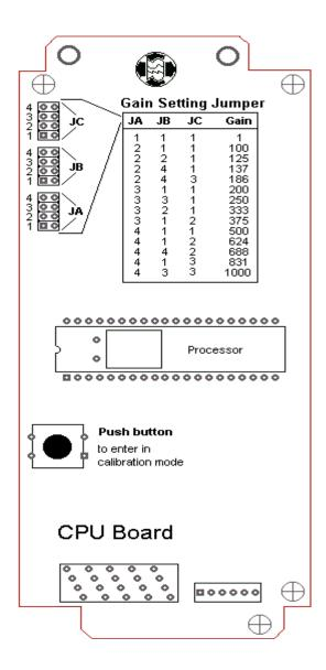
The gain setting is located on this board. Use 3 small jumpers to configure it. Default value is 333.
