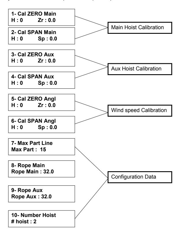
To enter into the calibration mode, unscrew the top cover to have access to the internal circuit. Turn the system on; wait until the system loads the basic screen display with load. Remove the "CAL" jumper located on the I/O Board. The system will alarm using the ATB light and buzzer. Press the push button located on the CPU Board.
