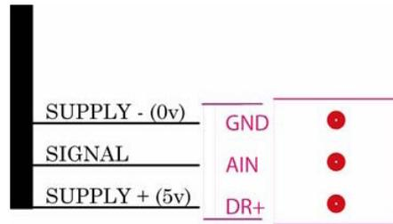
**Figure 2.6.3 – Three wire analog input**
