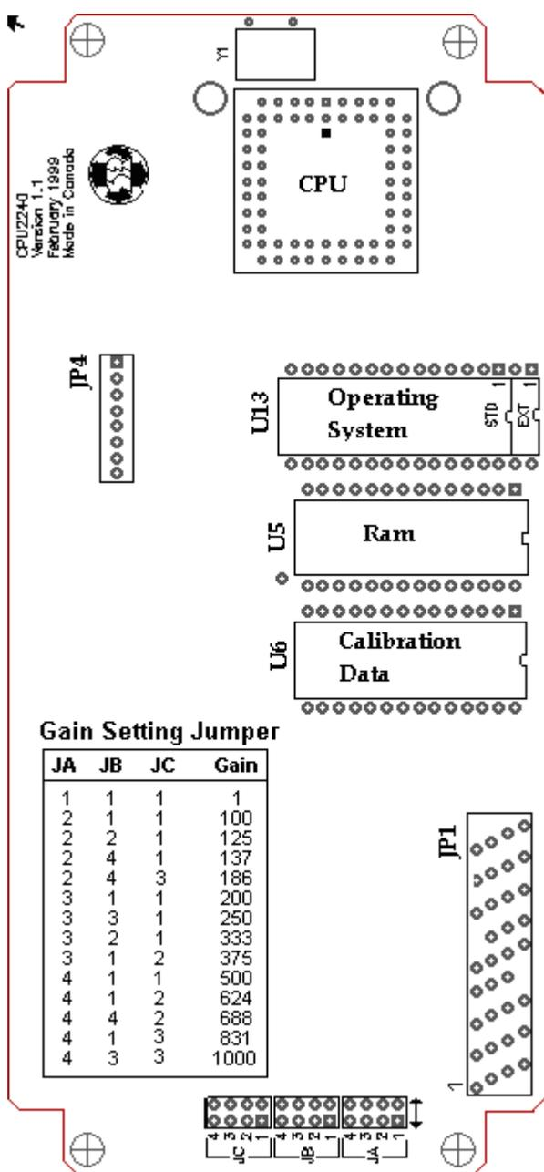
The Gain setting is located on this board, and are denoted JA,JB,JC. 3 small jumpers are used to configure it. The default value is 333
