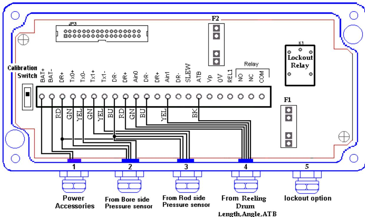
The lockout connection is according to your lockout configuration. Safe operation (without alarm) gives a relay status of COM-NO. When an ATB or Overload condition is detected, the relay status will change to COM-NC.
