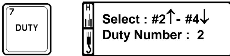
Pressing the duty button allows the duty number to be changed using buttons 2 and 4, note that the state of the optional slew sensor will affect the duty number and only those duties that are valid for the current slew sensor state will be displayed. Use enter (#1) or wait 15 seconds to confirm the selection.
