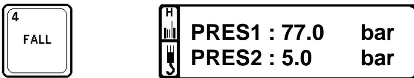
Pres1 is the full side pressure sensor and Pres2 is the Rod pressure sensor. The display reading is in bars.
