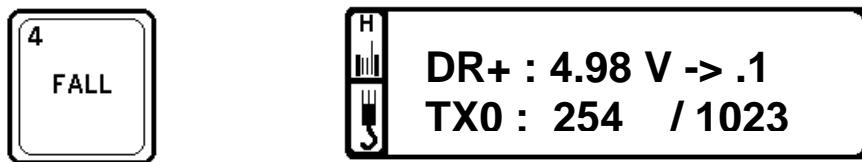
The DR+ is the sensor supply voltage. It normally indicates 5.00 Volts plus or minus 0.1 Volt. If the voltage is below 4.90 Volts, a sensor wire is shorted causing a drain of power. If the voltage is above 5.25 Volts, a load sensor wire is damaged or the internal amplifier is set incorrectly causing the load sensor voltage to increase above 4.95 Volts. A wrong DR+ will affect the readings on all sensors.
