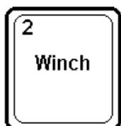
Used to select the Winch used. The secondary «UP» function is used to scroll up in menu or increase value being edited. This button will be referenced to this second function in this manual.
